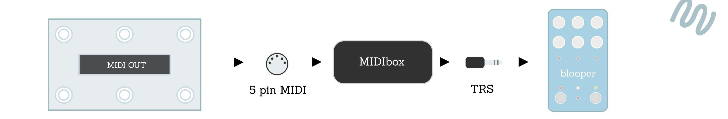
MIDI generally uses a unique 5-pin cable, but it can also be converted to TRS. That's what we need to do here. Chase Bliss makes a MIDIBox for this purpose. Ensure the MIDIBox is powered, connect the output from your controller to the MIDIBox's input, and connect a TRS cable from any of the MIDIBox's ¼" outputs to Blooper's MIDI input.
