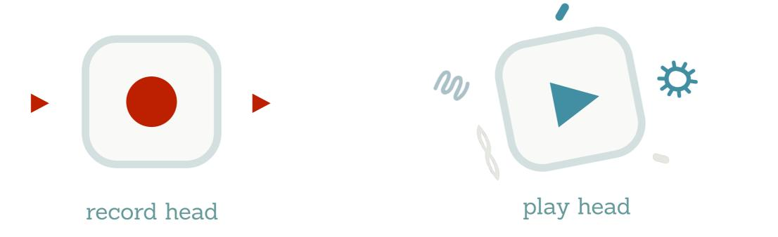
All loopers and delays use two different "heads" to achieve their effect. The name comes from tape machines – the record head puts sound information on to the tape, and the play head translates it back into sound. Even modern delays and loopers work like this, just without the tape.
